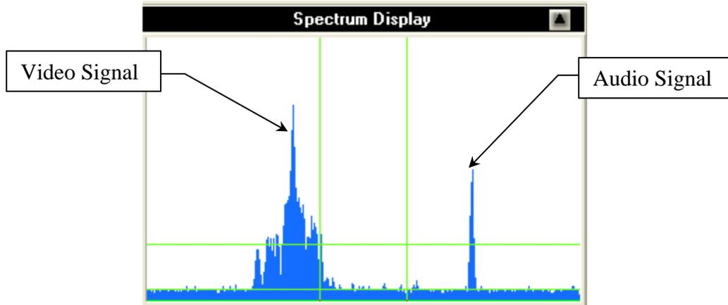
Commercial television broadcasts always have an audio signal transmitted at a frequency higher than the video (4.5 MHz higher for NTSC format and 6 MHz for PAL and SECAM formats). NTSC is the standard in North America and most of South America. Asia uses all three formats, depending on the country. European countries use PAL, except for France.
