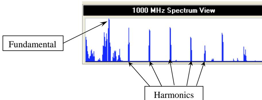
Harmonics are multiples of the original or fundamental frequency. For example, if a transmitter is at 120 MHz, harmonic signals will be seen every 120 MHz. So, you'll see them at 240, 360, 480 MHz and so on. They will show up as evenly spaced signals on the Scanned Spectrum Display. Five harmonics can be seen in the illustration. Sound from the eavesdropping transmitter will be heard on most or all of the harmonics during Audio Evaluation.
