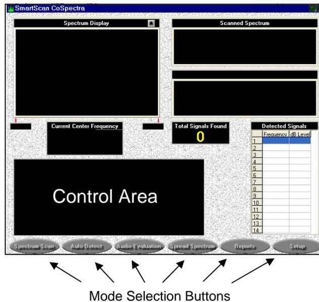
Across the bottom of the screen are 6 Mode Selection buttons. These are used to select the mode of operation for the required activity.
