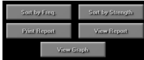
SmartScan offers different types of report formats. The first is as a listing of the frequencies and strengths of all of the detected signals. The second is a graphic representation of the RF spectrum that can show the entire spectrum up to a span of 1000 MHz or a selected portion as narrow as 10 MHz.
