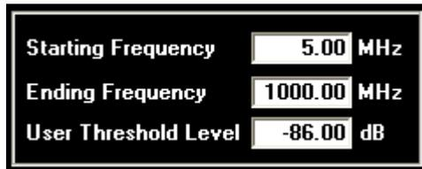
This is the frequency that the scan begins on. In AutoThreshold, User Threshold and Strong Signal Area Modes, the default starting frequency is 5 megahertz. The Starting Frequency for the Carrier Current Mode is 50 kHz (.05 MHz).
