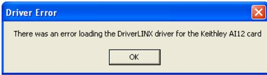
This error message indicates that the data acquisition card needed for AutoDetect mode is not present. It does not need to be installed unless AutoDetect mode will be used. If AutoDetect will not be used, click on OK. If AutoDetect mode will be
