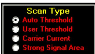
SmartScan has four different scan types operational in the Spectrum Scan mode: *User Threshold*, *AutoThreshold*, *Carrier Current*, and *Strong Signal Area*.
