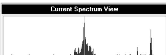
When evaluating a signal, there are times it is useful to see what the current display on the ECR looks like. When the **Current Spectrum** button is clicked, a 10 MHz slice of the spectrum based on the current center frequency will be shown in this display. With this display, the older signal can be compared to the
