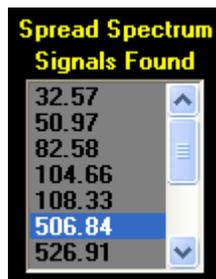
When the computer has completed the analysis of the scanned spectrum for signals that meet the criteria for spread spectrum transmissions, a list of frequencies appears here. The frequencies are the center frequencies of the detected signals.
