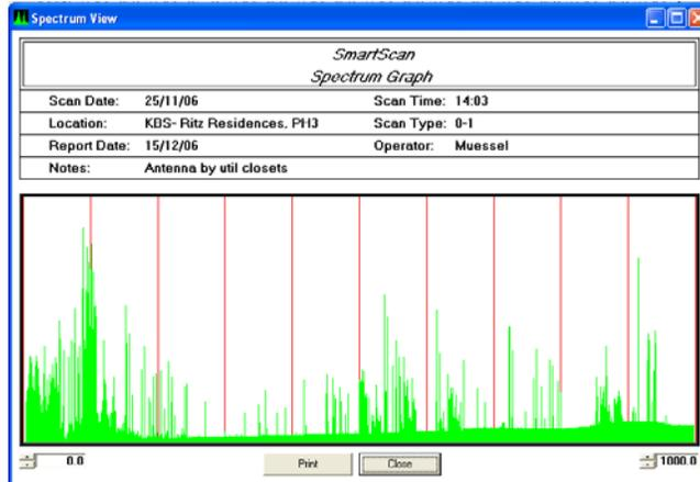
Note the numbers on the lower left and right corners of the graph. These show the frequencies of the edges of the report.
