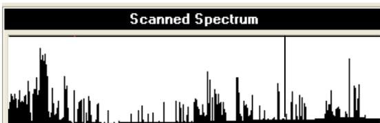
The Scanned Spectrum Display is a composite of all of the signals that were detected during the scan. It is like setting the display of the ECR to 1000 MHz with 9 kHz resolution bandwidth. It gives a snapshot of all of the signals that are on the air. The vertical red line indicates the position in the RF spectrum the ECR is tuned to.
