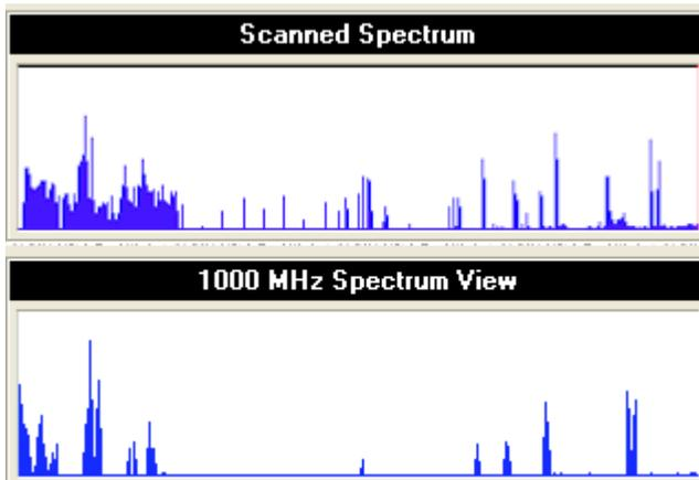
On the right-hand side of the computer screen are two smaller displays. The topmost display shows the entire spectrum as is it scanned. This display is built up 2 MHz at a time. The Scanned Spectrum Display shows signals as they are detected and it shows the progress of the scan.
