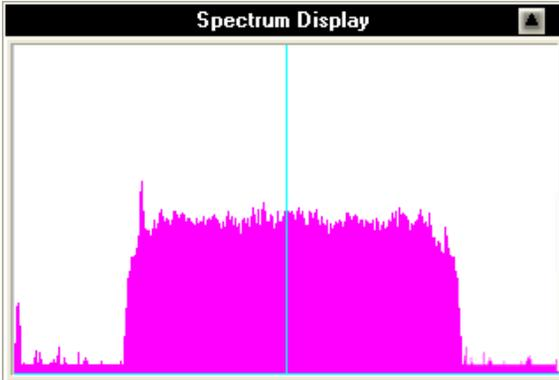
When in this mode, the display will show the selected spread spectrum signal. These signals frequently have a shape that looks like a mesa. It rises rapidly out of the noise floor and remains relatively flat across its span and then drops down quickly. Other spread spectrum signals will be more jagged and gradual in their rise and fall.
