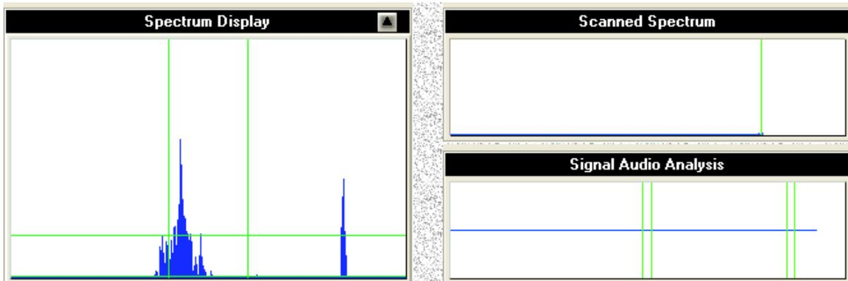
In the illustration above, note the two small detection windows on the Signal Audio Analysis display. These windows represent the location of the sounds from the SS3 sound source. If the frequencies are present, the signal will be added to the list.
