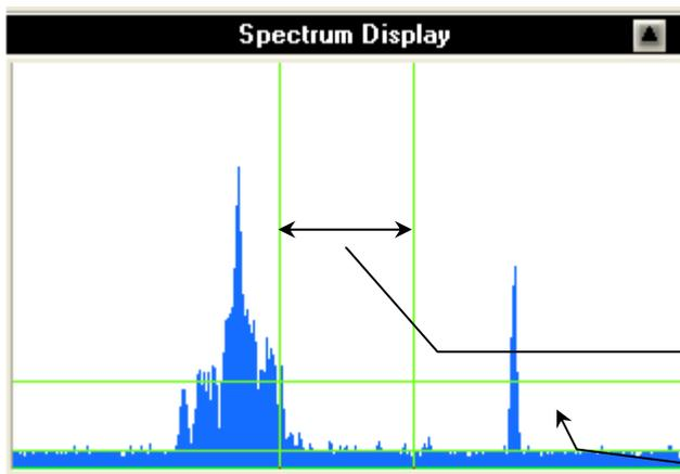
The Spectrum Display is an image of the ECR's spectrum display. It displays a window that shows 10 MHz of the RF spectrum. The display shifts in 2 MHz steps as the receiver scans across the spectrum. You will see signals appear on the right hand side of the display and move across to the left.
