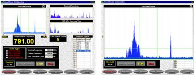
The button in the upper right hand corner of the display is to change the size of the Spectrum Display. Click on to increase the display to fill the width of the SmartScan program window.
