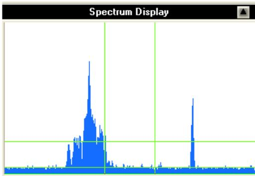
The spectrum display shown in Listen Mode is a composite of signals that were detected during the scan. It is not a real-time display. It shows the signals that were on the air and their amplitude when the scan was made.
