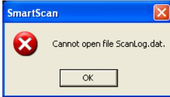
This error message occurs when you click on the **View ScanLog** button on the Scan Screen or when you click on **Compare Scans** in Audio Evaluation mode before any scans have been saved. SmartScan does not create the scan log file until it saves the first scan. Click **OK**. When the Scan Log window opens, click on Close and continue using SmartScan.
