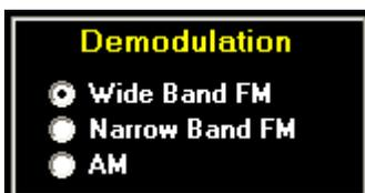
The ECR has two types of audio demodulation which are controlled by the computer: Wide and Narrow band FM and AM. FM is the default. Switching to the next or previous signal switches the demodulation to FM automatically.
